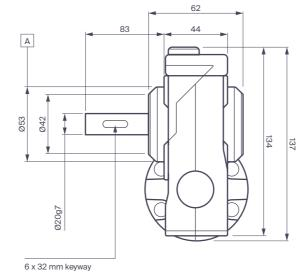
Technical data PM70-146 1 Motor 2 Voltage 12 - 48 V 3 Maximum power 220 W 4 Nominal speed 330 rpm 5.0 5 Nominal torque Nm 6 Peak torque Nm 22.0 7 Gearbox axial load 300 Ν Ν 500 8 Gearbox radial load 9 Gearbox efficiency 90 % 12.5 10 Gearbox ratio :1 11 Motor length mm 146
